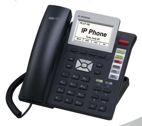
SIP-T65 is designed for maximum productivity and efficiency in the everyday business environment. Equipped with the TI TITAN chipset, SIP-T65 offers high definition voice quality through TI voice engine, HD handset, HD speaker and HD codec (G.722).
